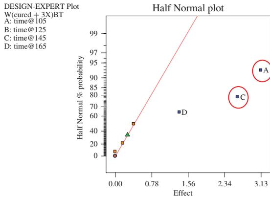
Fig. 6. Effects of VFM cure on die warpage.
