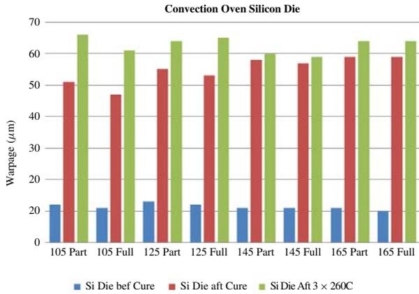
Fig. 3. BT Silicon die warpage with convection cure.
