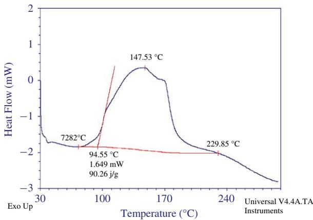
Fig. 10. DSC of un-cured UF8830.
