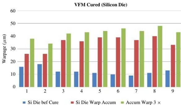
Fig. 8. Warpage results for silicon die side.
