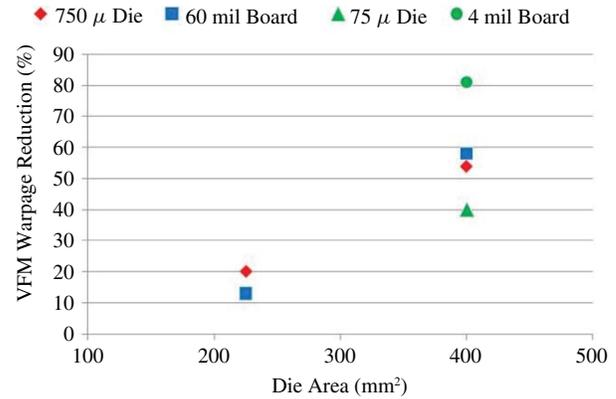
Fig. 16. VFM warpage reduction versus die size.
