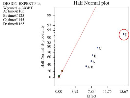
Fig. 5. Effects of VFM cure on BT warpage.
