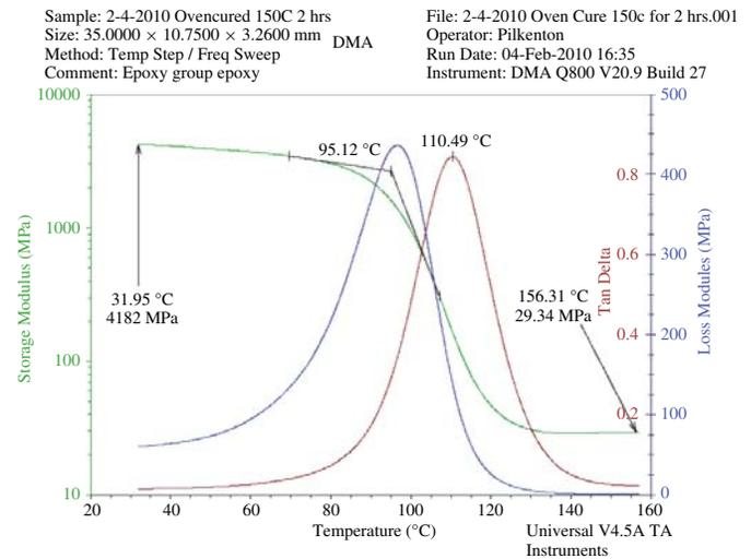
Fig. 17. DMA of UF8830—convection cured.
