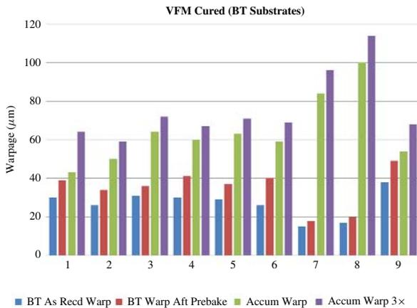
Fig. 7. Warpage results on BT substrates after cure.
