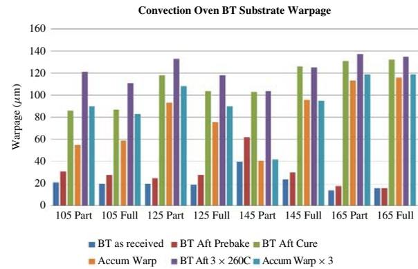
Fig. 2. BT Substrate warpage with convection cure.
