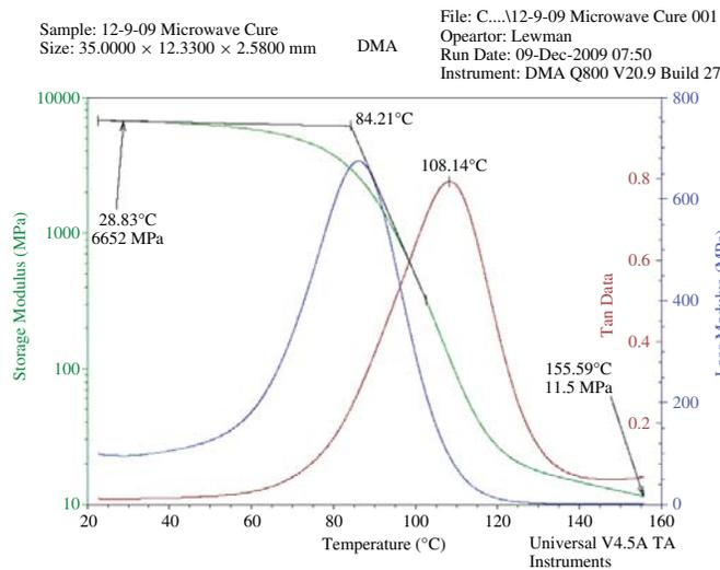
Fig. 18. DMA of UF8830—VFM cured.
