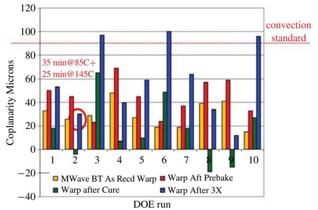
Fig. 14. BT substrate warpage for UF8830.
